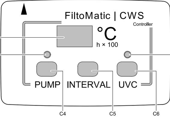
The diagram shows the control panel for the FiltoMatic | CWS system. It features a central display area with a temperature indicator (°C) and a 'Controller' label. Below the display are three buttons labeled 'PUMP', 'INTERVAL', and 'UVC'. To the right of the panel are three more buttons labeled 'C4', 'C5', and 'C6'. Lines connect these labels to their respective components in the diagram. A legend on the right side of the diagram explains the functions of each component.
